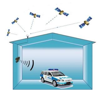
To use GNSS satellite devices inside your building you will need a repeater system to relay the signals from the outside to inside where there is no coverage. A repeater is a device that receives GNSS signals and retransmits them to the area required. This is achieved by connecting the repeater to an externally mounted antenna via a coaxial cable to its location inside the building.
