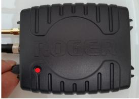
Constant green light indicates proper gain setting. Turning the knob too far counterclockwise will result in the green LED to blink indicating too low gain setting.
