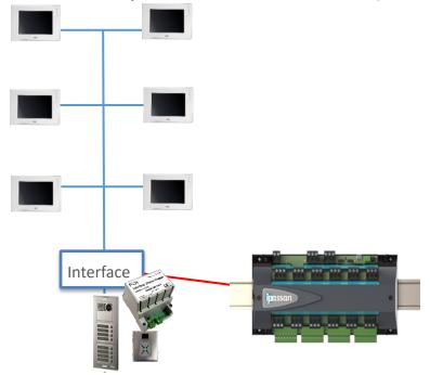
The 2Voice FDI integration is based on 2Smart door panels (FDI manufacturing). In this case, the complete interface features are available. In addition, the names on the entrance panels are managed in iPassan Manager. In that way, the building manager uses the software as a single access point for the access control of doors, floors and intercom.
