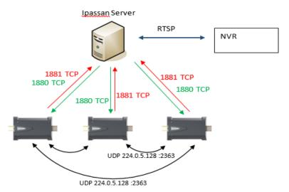
This integration works for live or replay. Note that when the NVR also supports the ONVIF protocol, iPassan Manager also allows you to control the PTZ (Pan Tilt Zoom) cameras from its supervision window.
