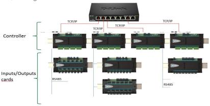
An access control network is limited to 32 Rs485 panels or 64 if the network contains IP. The network quantity is unlimited on iPassan, which lets you build freely.
